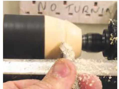
▲ Pic.11 As the tool makes its way through the shape, you will need to lift the handle as the wood gets smaller in diameter; this will maintain the bevel in contact with the wood
